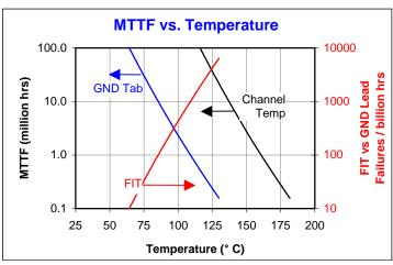
As can be seen from the MTTF values above, the predicted failure rate is still above 1 million hours, even at operating temperatures up to  $+110^{\circ}$  C (corresponding to channel temperatures of  $+162^{\circ}$  C). Also note that these MTTF estimates are a lower bound as the accelerated testing never resulted in 50% failures.
